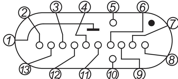
Pin numbering starts clockwise from the first pin, which is labeled on the component capsule by an arrow. The pin numbering scheme above is valid when the component is observed from the bottom.
